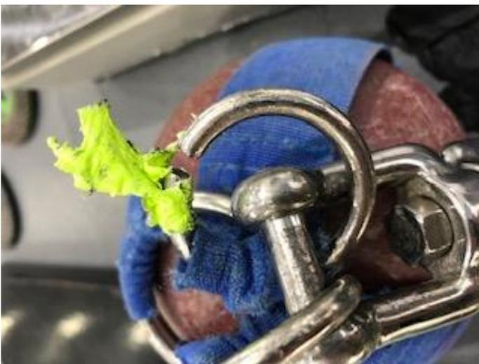
Tape was used to cover the broken ring. This shows why we should remove all tape before checking implements. Most tape is not allowed in any event. Although there is no picture, be sure to check the bolts holding these
