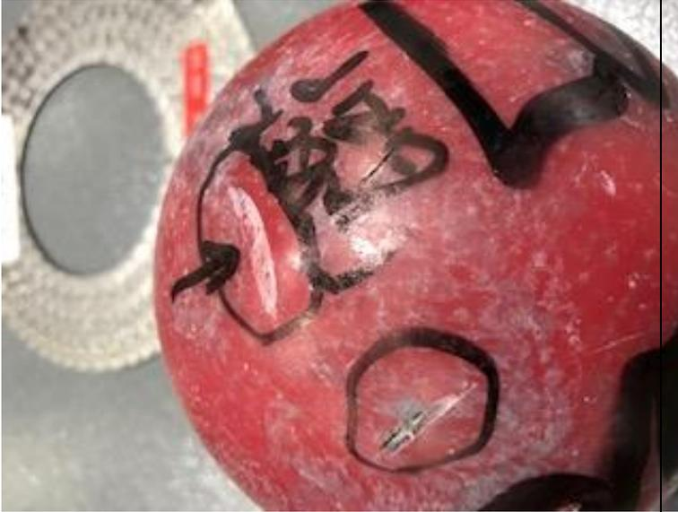
The following rubber ball is filled with lead shot but its shell is extremely soft and pliable. Its diameter also exceeds the indoor maximum for a 12 lb shot of 132.5 mm. This is an exercise ball, not a competition shot:
