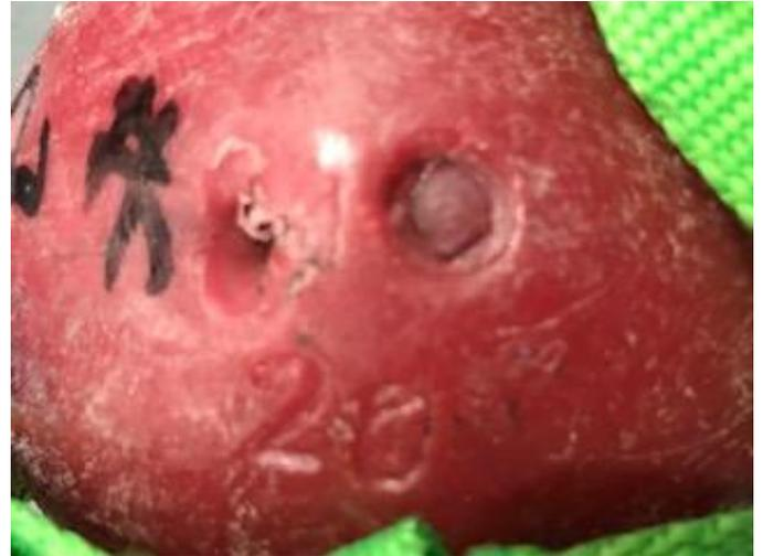
with some pretty big holes (indentations?). If those go deep enough, the lead fill can leak out and cause the shot to become light. If these are thrown onto a turf field, the lead pellets are toxic and need to be removed which is a major problem given the rubber pellets used as infill.
